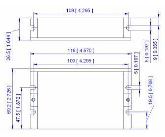
Figure 2-1: Mechanical specifications
