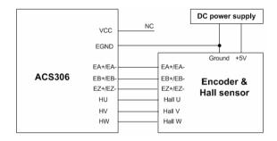
Figure 3-5: Using external DC power supply to supply the encoder
