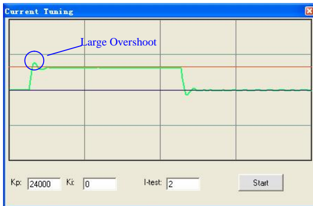
Figure 28: Response with High K_p of current-loop ( K_p = 24000 )
