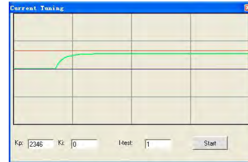
Figure 23: Kp=2346, Ki=0 (poor performances)
